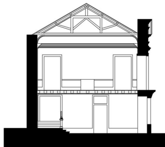
Fig. 30 transversal section through the building extension
