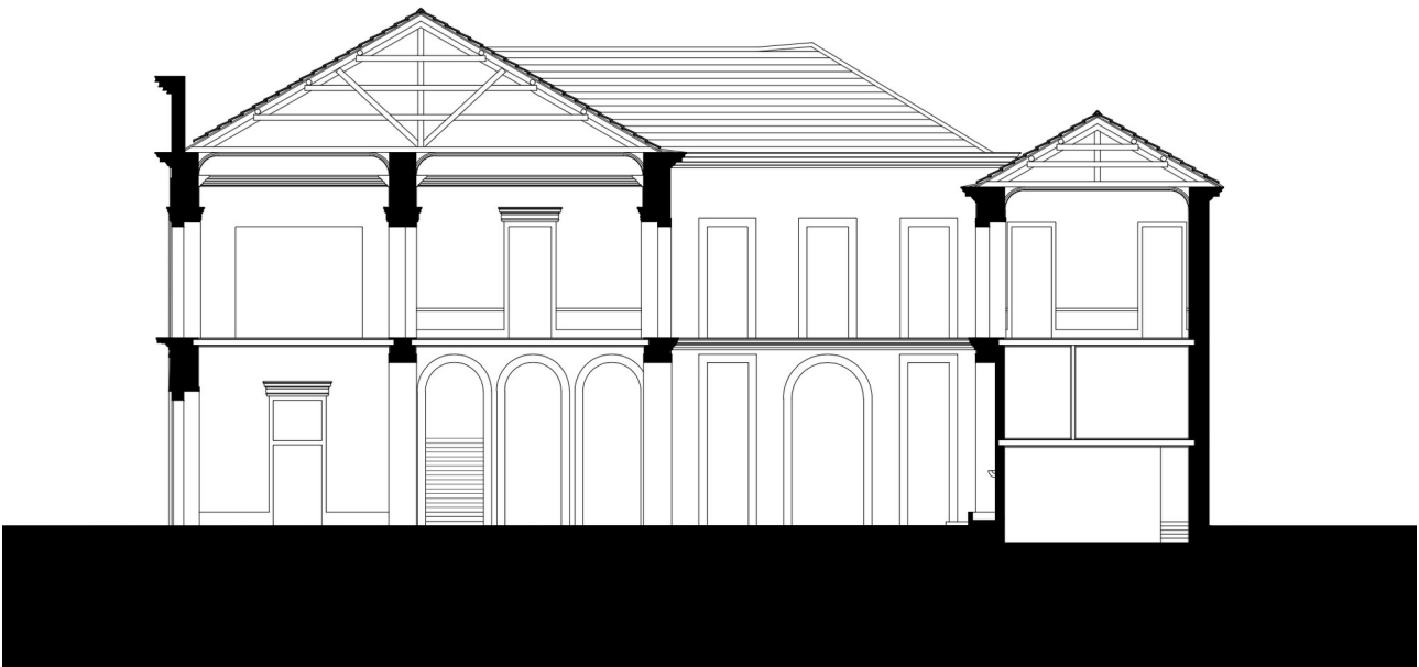
Fig. 31 section through the main building and patio
